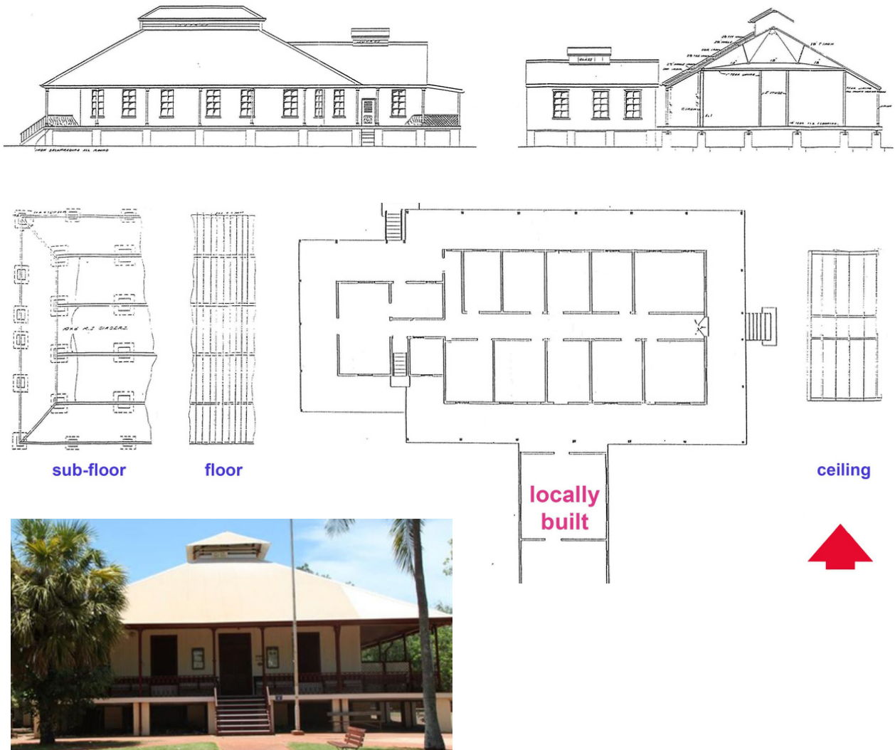
Broome Court House, former Cable Station: reconstruction plan: Miles Lewis, based principally upon 'Plan showing conversion of the Cable Station 1922', Department of the North West WA drg. no 108, PWD WA drg no 21441.
