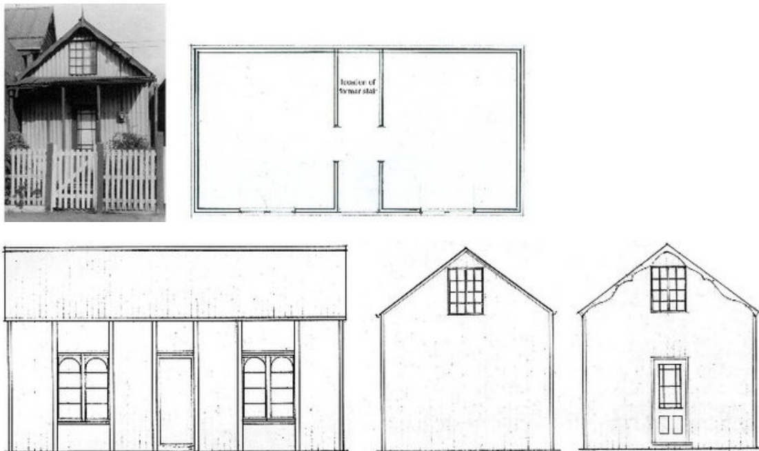
Iron cottage, Coventry Street (probably no 385, moved here c 1875, perhaps from the Patterson Place end of the site), view and survey as in 1959. Clare Lewis & Mary Lloyd, 'Portable Buildings' (BArch, University of Melbourne 1959), plates 29-31.
