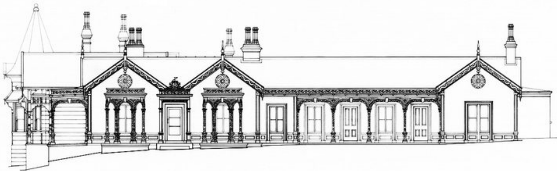
Corio Villa, Geelong, 1853-4, elevation, from a measured drawing survey by R Graham & M Krause, 1981, sheet 2, detail: State Library of Victoria H82.190/2. One curved portico has been moved northwards at the time of erection, and a square porch added at a later date. The Edwardian timber addition is visible at the left.
