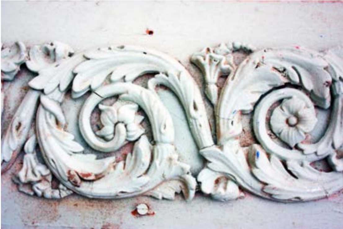
Wingecarribee, detail of papier mâché rinceau mounted on a board: Miles Lewis.
