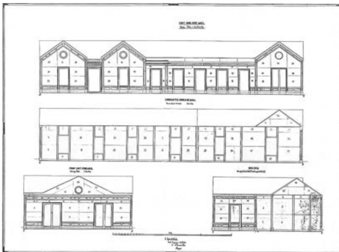
Bell & Miller's assembly drawing with 'cast iron side wall', 'corrugated iron side wall', 'front corrugated iron wall' and 'back view', copy signed 'N. R. McC.': courtesy of Ian Shearer [digitally restored].
