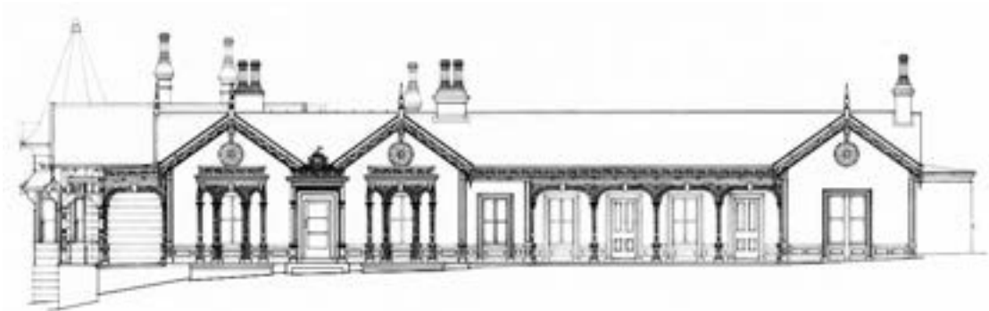
Corio Villa, Geelong, 1853-4, elevation, from a measured drawing survey by R Graham & M Krause, 1981, sheet 2, detail: State Library of Victoria H82.190/2. One curved portico has been moved northwards at the time of erection, and a square porch added at a later date. The Edwardian timber addition is visible at the left.
